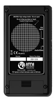
The IMI Inspector Alert<sup>TM</sup> V2 measures alpha, beta, gamma and x-radiation using a 2-inch "pancake" GM detector with high sensitivity to common beta and alpha sources. The easy-to-read digital display shows readings in your choice of  $\mu$ Sv/hr, mR/hr, CPM, or CPS. The Total/Timer feature allows timed readings from one minute to 40 hours for precise measurement of low level contamination. An audible alert sounds when the radiation reaches a user-adjustable level.
